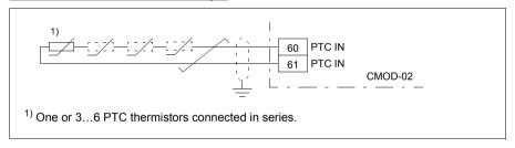
The PTC input is reinforced/double insulated. If the motor part of the PTC sensor and wiring are reinforced/double insulated, voltages on the PTC wiring are within SELV limits.
